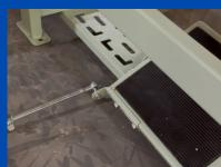
Attach balljoint rod to treadle extension.
