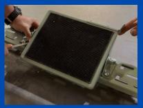
Slide treadle between lugs. Push lugs flush against treadle. Tighten lug screws to lock treadle in place.
